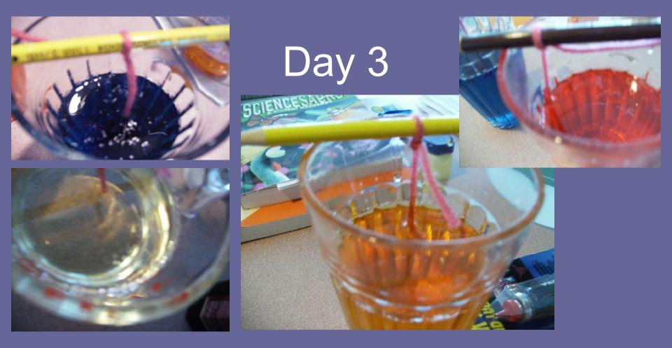
Greater crystal formation was evident by Day 3. The blue solution was crystallizing at the bottom of the wick and on top of the solution and glass. Tiny, translucent crystals appeared to be forming on the yellow and red wick, while the crystals were growing only on the glass that contained the controlled solution.
