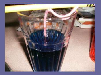
It was hard to capture the changes in the glasses because of the size of the crystals that were forming. The crystals were growing on the surface of the solution and up the side of the glass. The yellow solution appeared to saturate it's wick and develop a shiny crust that could be the beginning of sugar crystals.
