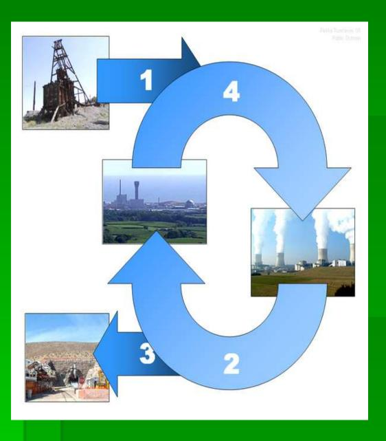
The nuclear fuel cycle begins when uranium is mined, enriched, and manufactured into nuclear fuel, (1) which is delivered to a nuclear power plant. After usage in the power plant, the spent fuel is delivered to a reprocessing plant (2) or to a final repository (3) for geological disposition. In reprocessing 95% of spent fuel can be recycled to be returned to usage in a power plant (4).
