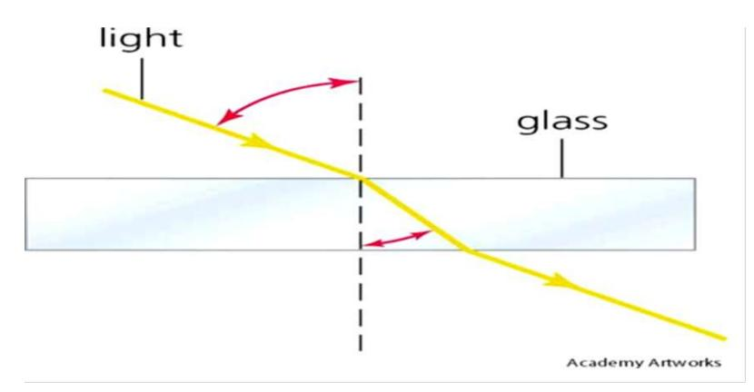
Refraction is what gives the illusion of a bent straw or spoon in a clear glass of water.
