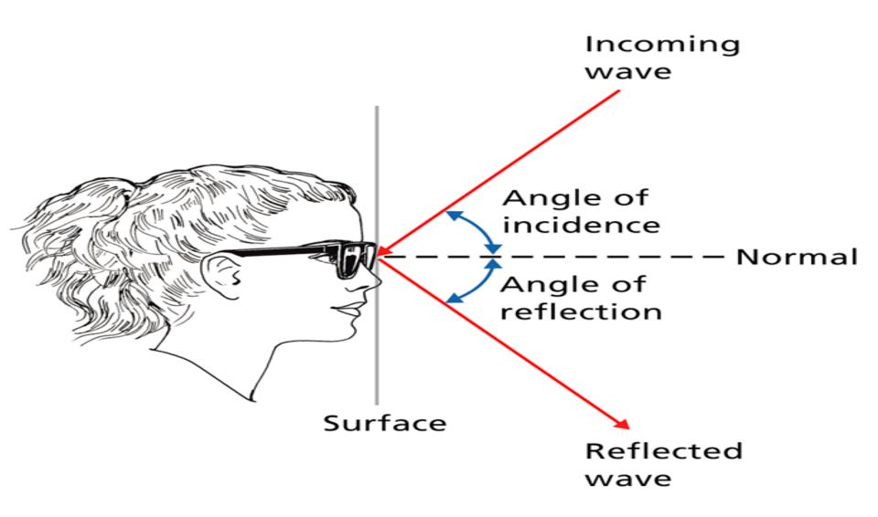
Notice: the angle with which the ray of light hits the surface is the same with which the ray of light is **reflected**
