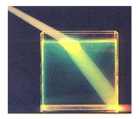
Refraction at the water surface gives the "broken pencil" effect.
