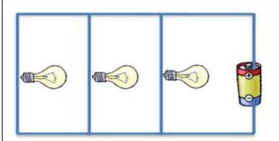
Justification: Parallel circuit: There are three paths for the current to pass through. If one circuit is broken, the other lights will still illuminate.
