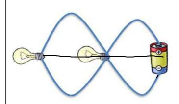
Justification: Parallel circuit: There are two paths for the current to pass through. If one circuit is broken, the other light will still illuminate.
