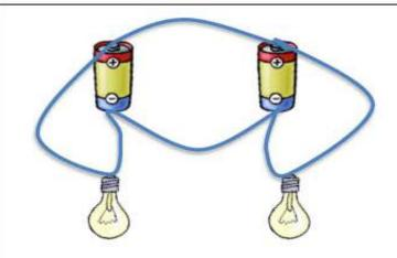
Justification: Parallel circuit: There are two paths for the current to pass through. If one circuit is broken, the other light will still illuminate.
