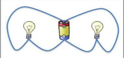
Justification: Two series circuits: There is only one path for the current to pass through to each light. If there is a break in the circuit to one of the lights, the affected light will go out.
