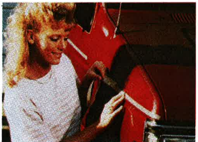
Figure 20-8 Plastic pinstripes being applied to this vehicle. (Spartan International)
