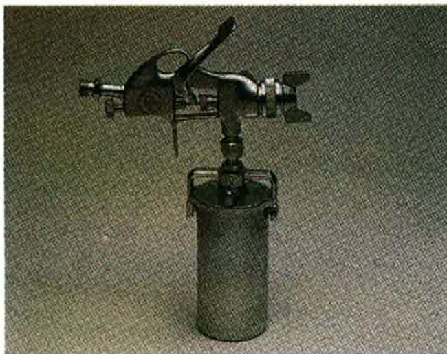
Figure 20-2 A touch-up gun is commonly used for spot repairs. Note the size of the paint container. (The Eastwood Co.)
