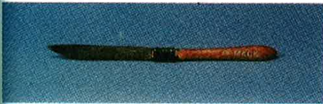
Figure 20-5 A typical brush used for applying painted pinstripes. (The Eastwood Co.)
