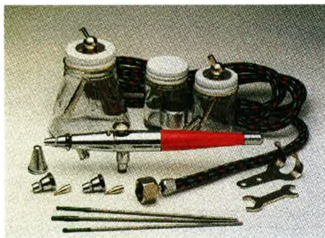
Figure 20-3 An air brush is used for fine detail work. This tool does not have a spray pattern control. (The Eastwood Co.)
