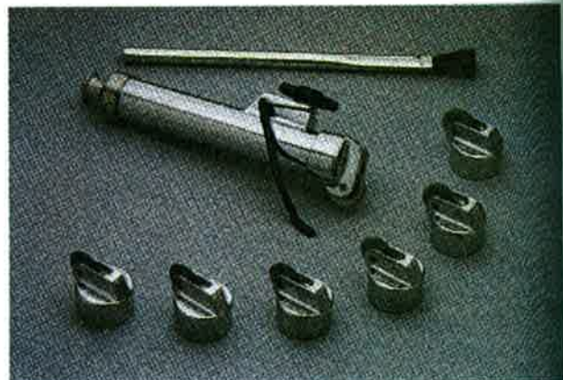
Figure 20-4 This striping tool is used when painting pinstripes. (The Eastwood Co.)
