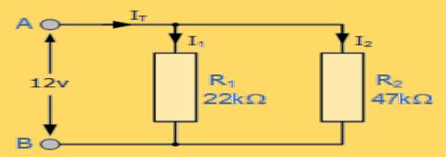
The Equivalent Resistance of a circuit with two resistors in parallel is given by
