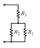
In this circuit,  $R_1$  and  $R_2$  are in parallel and  $R_3$  is in series with the combo set of  $R_1$  and  $R_2$
