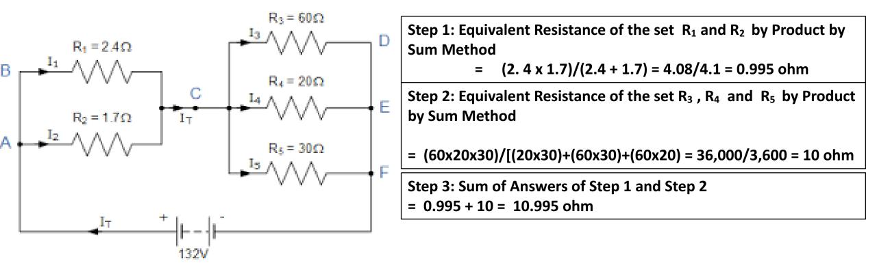
Determine the Equivalent Resistance of the following circuit; Show complete work
