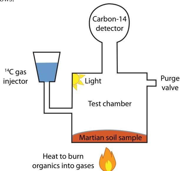
Figure 3. Set-up of PR experiment.
