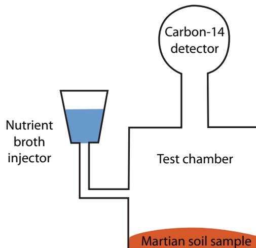
Figure 1. Set-up of LR experiment.
