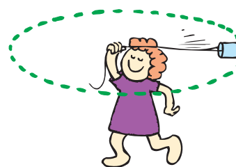
FIGURE 10.8 ▲ The force exerted on a whirling can is toward the center. No outward force acts on the can.
