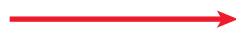
FIGURE 5.1 ▲ This vector, scaled so that 1 cm = 20 km/h, represents 60 km/h to the right.
