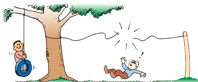
FIGURE 2.14 ► You can safely hang from a clothesline hanging vertically, but you'll break the clothesline if it is strung horizontally.
