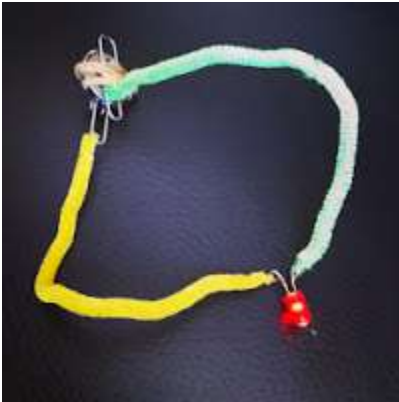
The simple circuit: two pipe cleaners (with ends stripped of fuzz), one LED light (with legs curled), two paper clips, rubber band and disc battery
