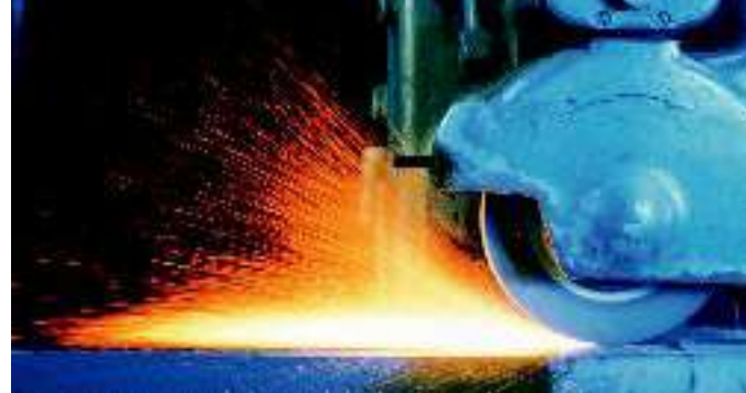
Figure 9.13 A grinding wheel made of silicon carbide ( \text{SiC} ) can shape even the toughest materials. Inferring What causes the sparks?
