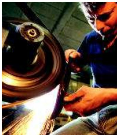
Figure 8.29 Silicon carbide, a network solid, is so hard that it is used in this grindstone to wear down the end of a hardened steel cutting tool to form a sharp edge.
