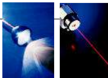
Flashlight beam vs. laser beam Light from a flashlight travels in different directions, covering a wide area. Light rays from a laser travel parallel to one another, resulting in a narrow beam of intense light in a specific direction.
