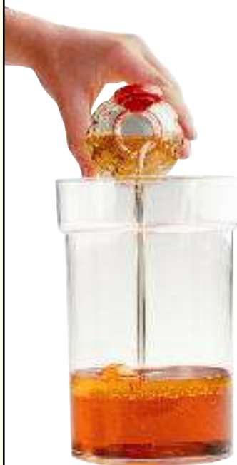
Figure 3.14 Because of differences in density, corn oil floats on top of corn syrup.
