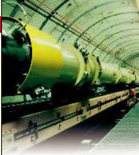
Figure 25.9 Fermilab is a major accelerator center located in Batavia, Illinois. The main accelerator is a ring that has a radius of 1.0 km.
