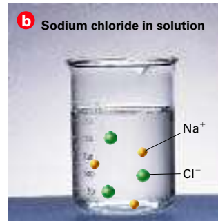
b Three moles of sodium chloride dissolved in water produce 6 mol of particles because each formula unit of NaCl dissociates into two ions.
