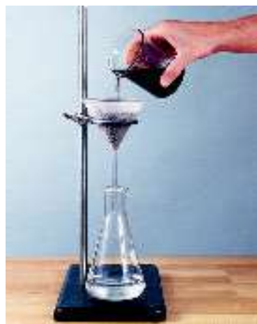
Figure 15.14 A suspension is a heterogeneous mixture. Suspended particles can be removed by filtration. Comparing and Contrasting How does the filtration of a suspension compare with the filtration of a solution?
