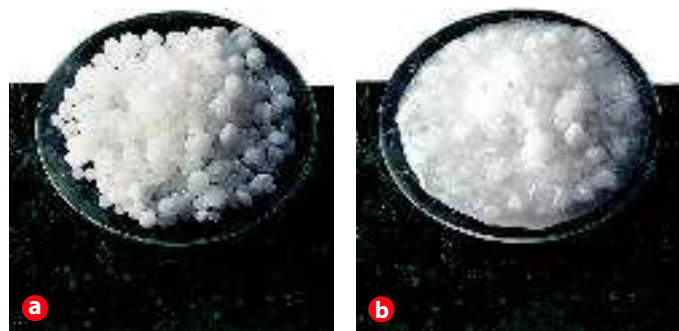
Figure 15.13 Deliquescent substances can remove water from the air. a Sodium hydroxide pellets absorb moisture from the air. b Eventually a solution is formed. Applying Concepts Identify the solvent and the solute.
