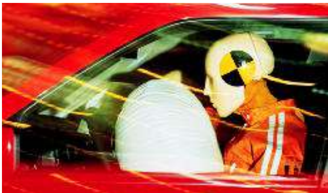
Figure 14.1 A crash dummy can be used to test the effectiveness of an air bag. Because gases can be compressed, the air bag absorbs some of the energy from the impact of a collision. Air bags work best when combined with seat belts.
