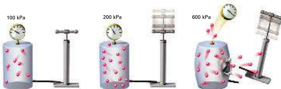
Figure 14.4 When a gas is pumped into a closed rigid container, the pressure increases as more particles are added. If the number of particles is doubled, the pressure will double.
