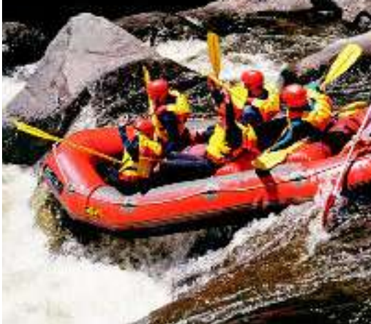
Figure 14.3 The volume of this air-filled raft is much larger than its volume before it was inflated. Using a pump to force air into a raft increases the pressure of the air inside the raft. The increased pressure causes the raft to inflate to its intended size.
