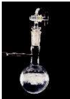
Figure 13.16 At the triple point, ice, liquid water, and water vapor can exist at equilibrium. Freezing, melting, boiling, and condensation can all occur at the same time, as shown in the flask.
