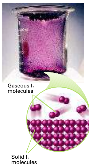
Figure 13.14 When solid iodine is heated, the crystals sublime, going directly from the solid to the gaseous state. When the vapor cools, it goes directly from the gaseous to the solid state.
