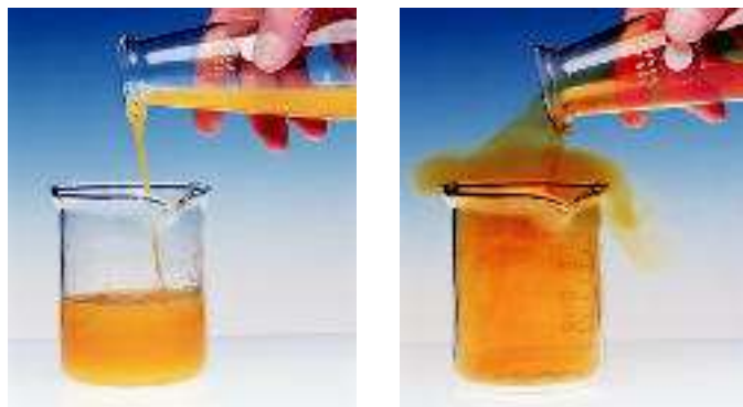
Figure 13.5 Both liquids and gases can flow. The liquid on the left is colored water. The gas on the right is bromine vapor. If a gas is denser than air, it can be poured from one container into another. These pictures were taken in a fume hood because bromine is both toxic and corrosive.
