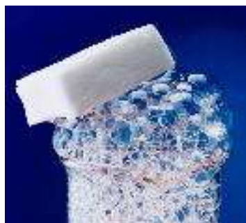
Figure 1.7 This insulation is light enough to float on soap bubbles yet is very effective at preventing heat transfer.
