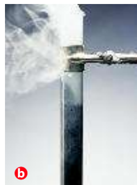
Figure 11.3 Hydrogen peroxide decomposes to form water and oxygen gas. a Bubbles of oxygen appear slowly as decomposition proceeds. b With the addition of the catalyst manganese(IV) oxide ( \text{MnO}_2 ), decomposition speeds up. The white "smoke" is condensed water vapor.
