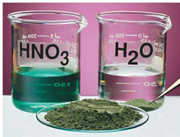
\text{NiO} is insoluble in water but reacts with \text{HNO}_3 to give a green solution of the salt \text{Ni}(\text{NO}_3)_2
