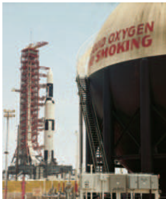
Figure 6 Rockets differ according to the types of fuel used to launch them. Liquid oxygen is used often to support combustion.
