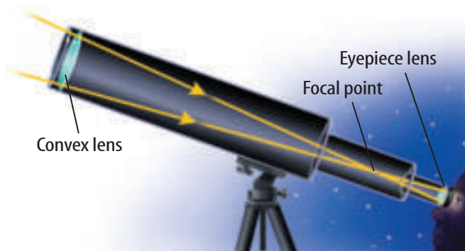
Figure 2 These diagrams show how each type of optical telescope collects light and forms an image.
