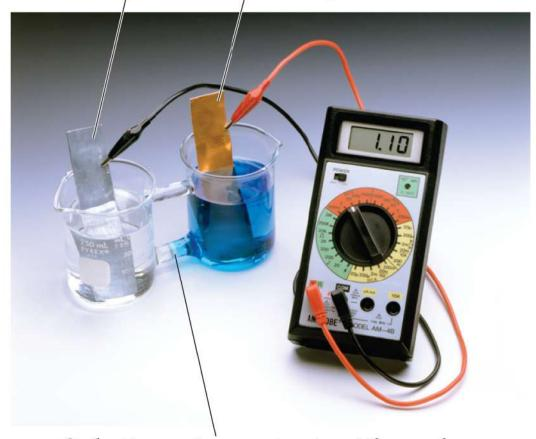
Solutions in contact with each other through porous glass disc
