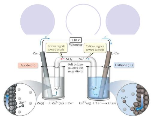
• How is electrical balance maintained in the left beaker as Zn<sup>2+</sup> is formed at the anode?
