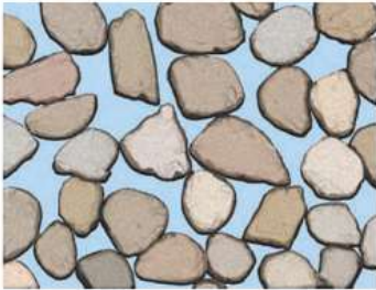
Well-sorted, coarse-grained sediment has high porosity.
