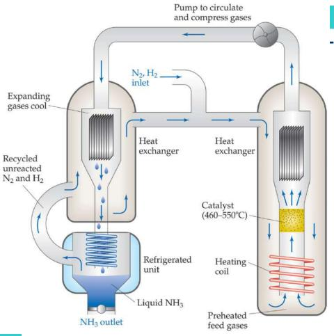
This apparatus helps push the equilibrium to the right by removing the ammonia (NH<sub>3</sub>) from the system as a liquid.
