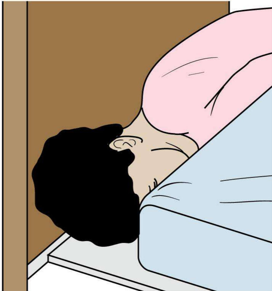
Fig. 14-10. Hospital bed system entrapment zones. G, Zone 7: Between the headboard or footboard and the end of the mattress.
