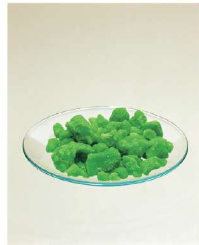
\text{NiCl}_2 \cdot 6 \text{H}_2\text{O}(s) remains when solvent evaporated
