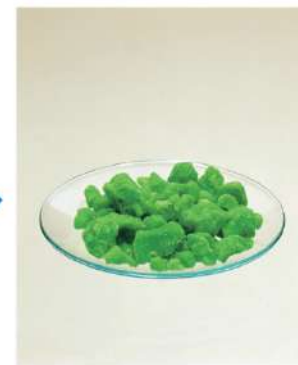
\text{NiCl}_2 \cdot 6\text{H}_2\text{O}(s) remains when solvent evaporated
