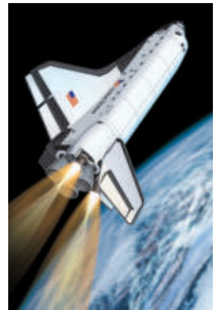
Figure 6 Wings help move aircraft in lower layers of the atmosphere. The space shuttle can't use its wings to maneuver in the exosphere because so few molecules are present.
