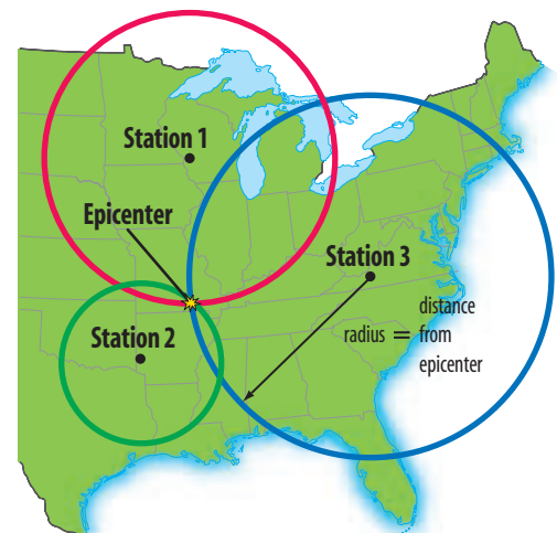
Figure 12 The radius of each circle is equal to the distance from the epicenter to each seismograph station. The intersection of the three circles is the location of the epicenter.
