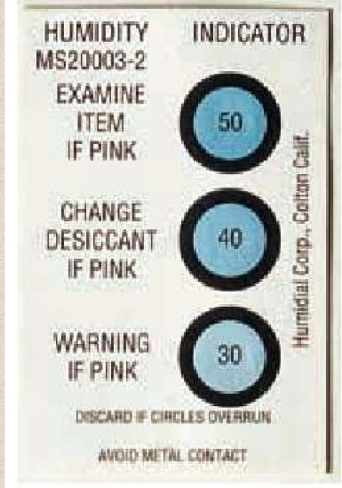
This humidity detector uses cobalt (II) chloride, CoCl<sub>2</sub> · 6 H<sub>2</sub>O.
