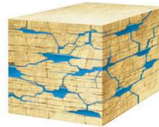
Rock is considered permeable if its empty spaces are connected so that water may flow from one space to the next.
