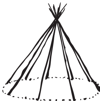
Step 2: Bind six poles to the tripod.
