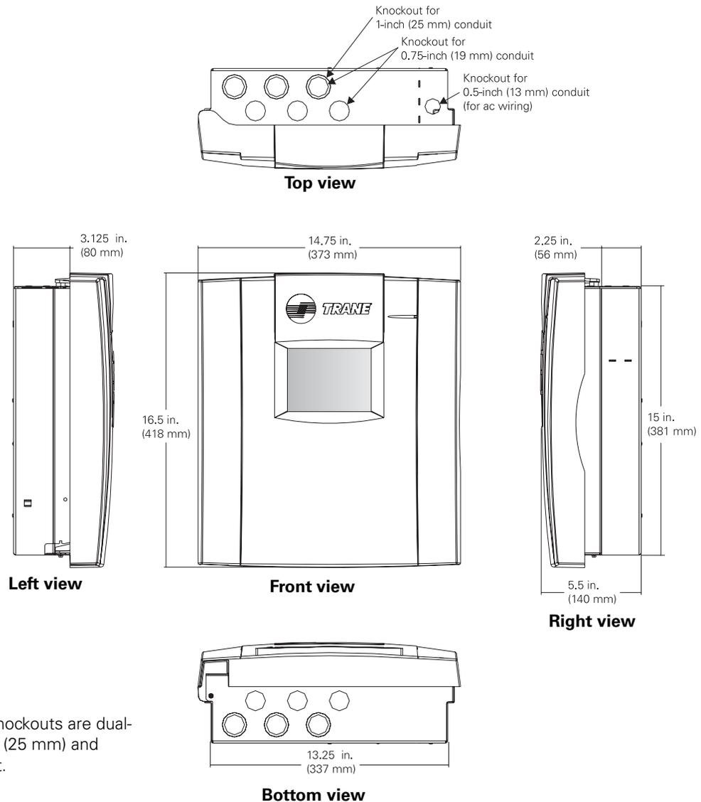
**Note:** Six of the twelve knockouts are dual-sized knockouts for 1-inch (25 mm) and 0.75-inch (19 mm) conduit.
