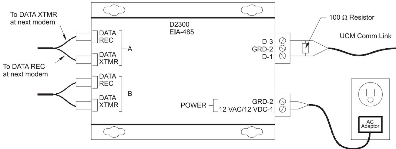
To mount and wire a D1300 and/or D2300 modems on an inter-building communication link, follow these procedures (see Figure 21 on page 41):
