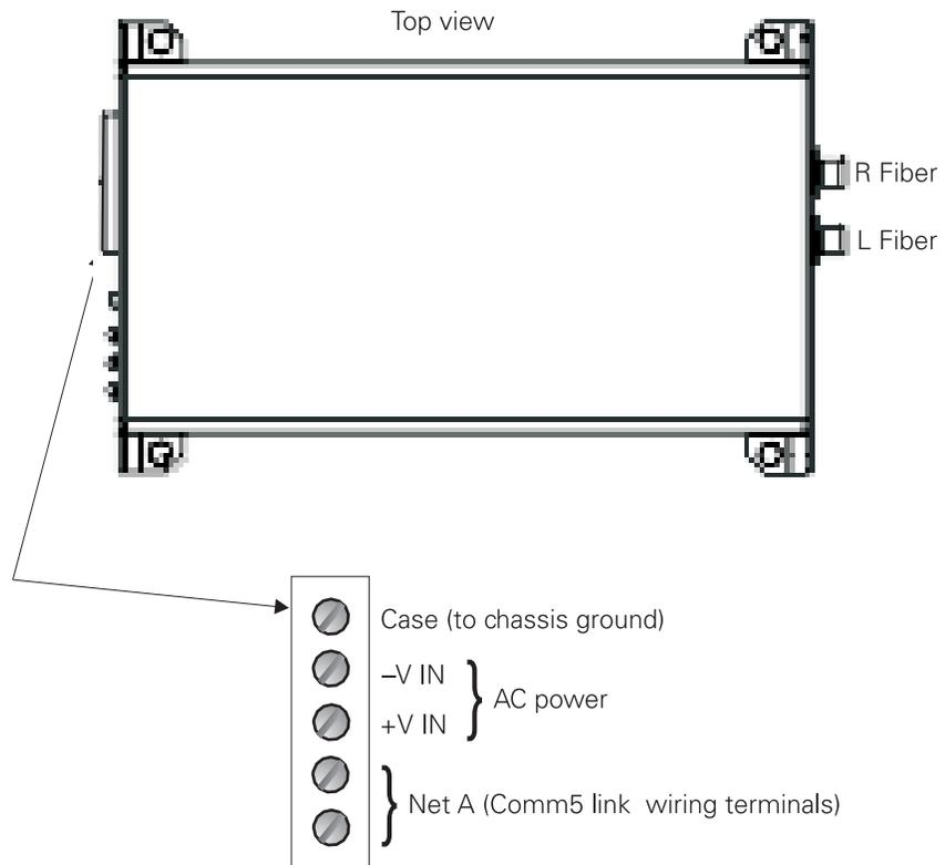
To mount and wire CBL 75090-4 modems on an inter-building communication link, follow these procedures (see Figure 26 on page 52):
