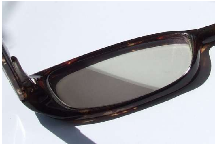
Figure 5: Photochromic lens partially exposed to sunlight
