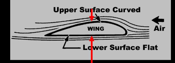
Air flows faster over the top – pressure is lower Net Force is upward
