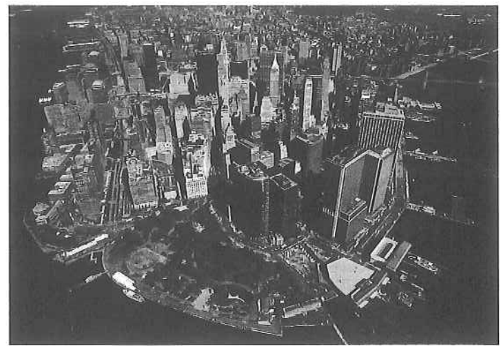
FIGURE 1-10 Changing site of New York City. Much of the southern part of New York City's Manhattan Island was built on landfill. Several times in the past 200 years, the waterfront has been extended into the Hudson and East rivers to provide more land for offices, homes, parks, warehouses, and docks. The World Trade Center was built during the late 1960s and early 1970s partially on landfill in the Hudson River from the colonial era. Battery Park City (at left in the photograph) was built on landfill removed from the World Trade Center construction site. Excavating the landfill from the World Trade Center site unearthed a large number of maritime objects, such as anchors, because the site was underwater in the seventeenth century.
