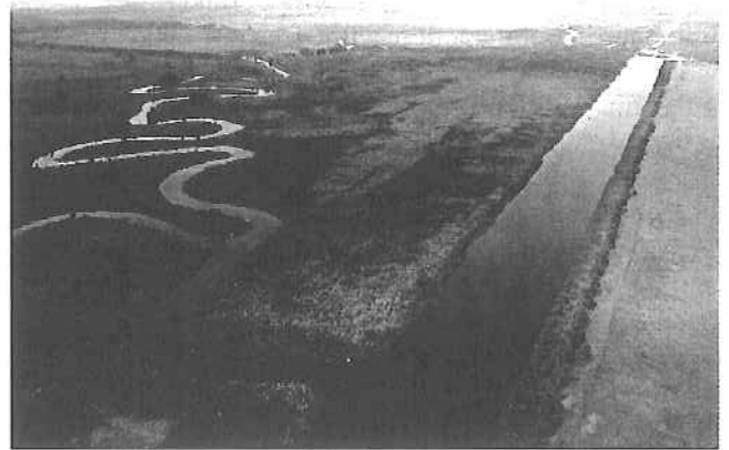
FIGURE 1-22 Environmentally insensitive cultural ecology in Florida. To control flooding in central Florida, the U.S. Army Corps of Engineers straightened the course of the Kissimmee River, which had meandered for 160 kilometers (98 miles) from near Orlando to Lake Okeechobee. The water was rechanneled into a canal 90 meters wide (300 feet) and 9 meters deep (30 feet), running in a straight line for 84 kilometers (52 miles). After the canal, known as C-38, opened in 1971, millions of gallons of polluted water—mainly runoff from cattle grazing—began pouring into Lake Okeechobee, which is the major source of freshwater for about half of Florida's population. The U.S. Army Corps of Engineers has returned the river from the canal (on the right side of the photograph) to its original course (on the left side).
