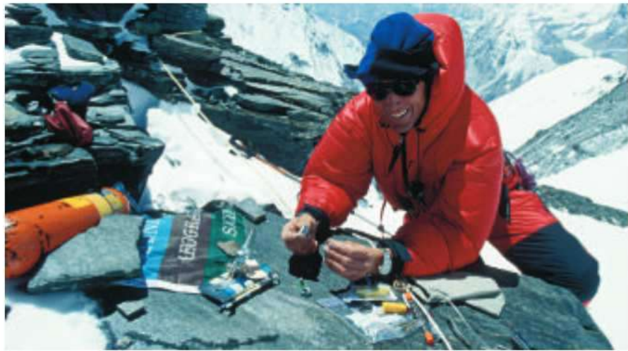
■ Figure 1-14 A series of expeditions succeeded in placing a GPS receiver on top of Mount Everest. This improved the accuracy of the altitude measurement: Everest's peak is 8850 m, not 8848 m, above sea level.
