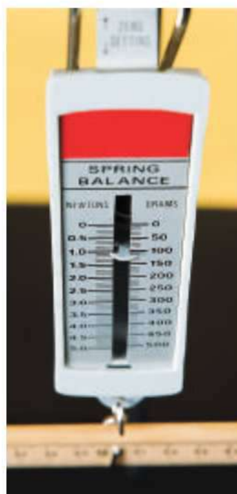
■ Figure 1-13 By positioning the scale head on (a), your results will be more accurate than if you read your measurements at an angle (b). How far did parallax shift the measurement in b?
