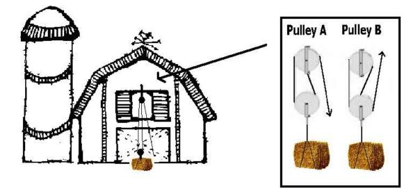
Describe the advantages of using <u>each</u> pulley system to assist the brothers in their decision-making process for this task.
