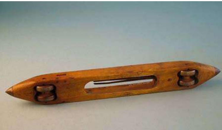
Shuttles like these had sharp, pointed ends that could cause serious damage if they flew off the loom, as happened all too often
