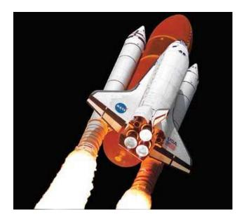
A good example is the space shuttle, as the shuttle loses fuel and jettisons it's solid rocket boosters it therefore loses mass. If the mass DECREASES, the acceleration INCREASES provided the FORCE (of thrust) remains constant.
