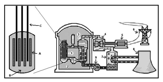
The process by which a nuclear reactor converts the heat released by a nuclear fission reaction into electricity.
