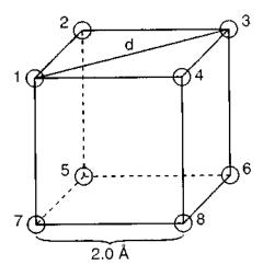
In the cubic crystal shown, if each edge is 2.0 angstroms in length, what is the diagonal distance, d, between atoms 1 and 3? (Assume that the Pythagorean theorem can be used to solve this problem.)
