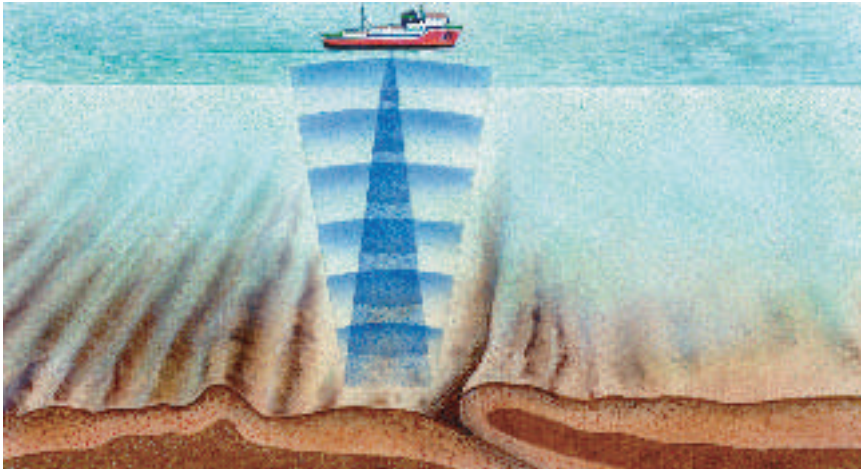
Figure 7 Sonar uses reflected sound waves to determine the location and shape of an object.
