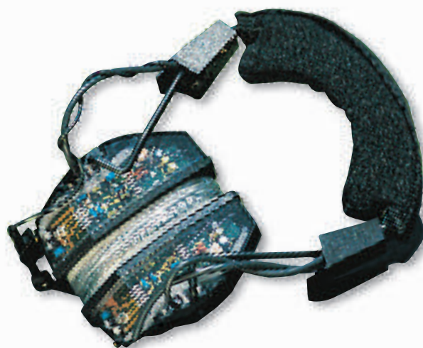
Figure 17 Some airplane pilots use special ear protectors that cancel out engine noise but don't block human voices.
