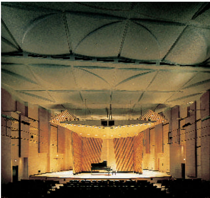
Figure 21 The shape of a concert hall and the materials it contains are designed to control the reflection of sound waves.
