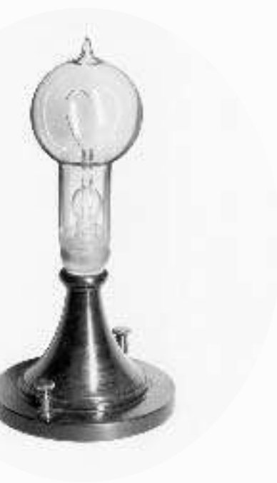
Figure 3 Edison designed an airless glass bulb in which to test filament materials.
