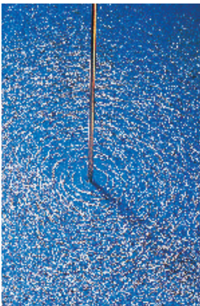
Figure 4 Electrons moving in a wire produce a magnetic field in the surrounding space. This field causes iron filings to line up with the field.
