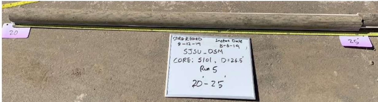
Photo: Sample Core Run, column S101 run 5
