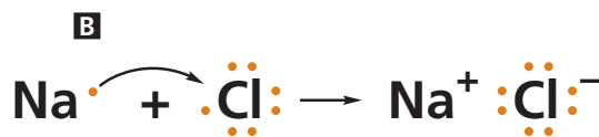
Figure 5 A When sodium metal comes in contact with chlorine gas, a violent reaction occurs. B Sodium atoms transfer one electron to the outer energy levels of chlorine atoms. Both ions now have filled outer energy levels C The positive and negative ions formed attract each other to form a crystalline solid with a rigid structure.
