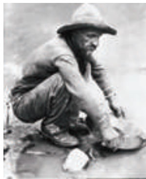
Figure 8 Placer deposits led to the California gold rush. Here, a prospector in 1850 swirls his gold pan, separating sand and mud from flecks of gold.
