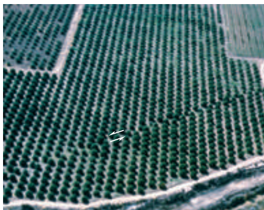
Figure 3 Slippage along a fault caused an offset in this orange grove east of Calexico, California. The white arrows show the direction of movement on either side of the fault.
