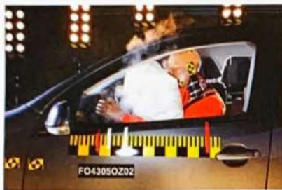
▲ Figure 3.7 Decomposition of sodium azide, \text{NaN}_3(s) , is used to inflate air bags in automobiles.
